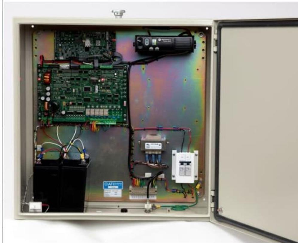
Figure 7. Onsite Remote Terminal Unit [15]
